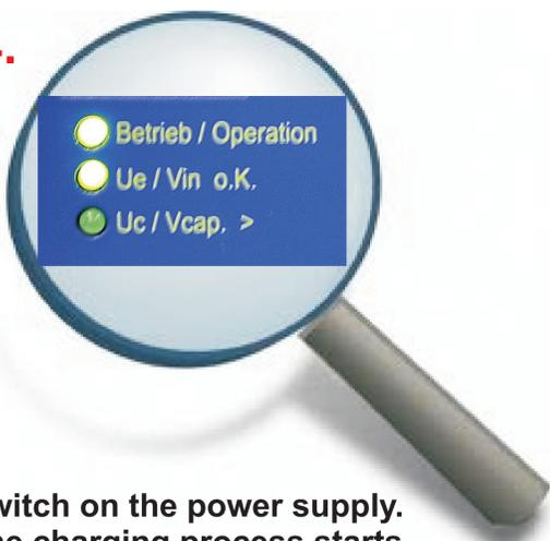
Switch on the power supply. The charging process starts. The LEDs „Betrieb/Operation“, and „U<sub>e</sub>/V<sub>in</sub> o.K.“ illuminate
