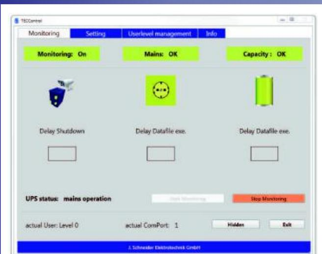
The *TECCentral*-Software automates the system-shutdown at power failure and the controlled system-restart after power recovery.
