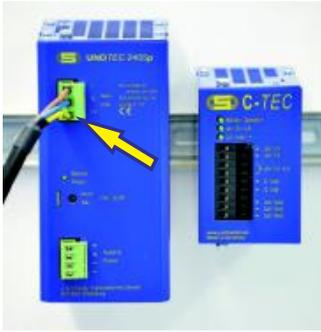
Connect the 24 V DC power supply to the mains (230 V AC)
