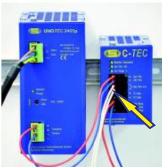
Wiring of the signal contact. Input voltage OK
