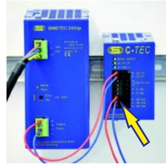
Connect the load to the buffered 24 V DC output of the C-TEC
