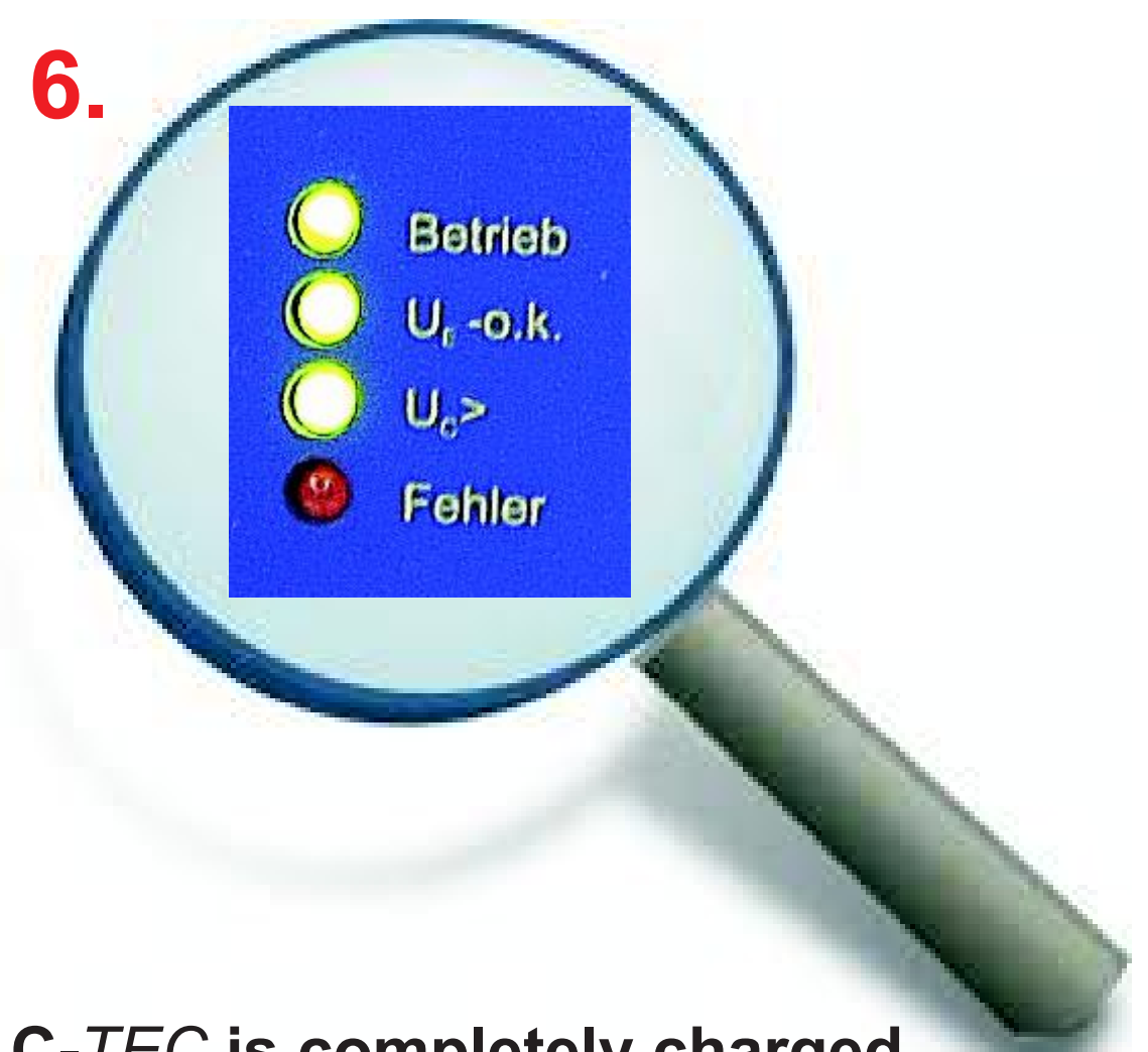
6. C-TEC is completely charged. The LEDs „Betrieb“, „U E ok“ and „U C >“ illuminate
